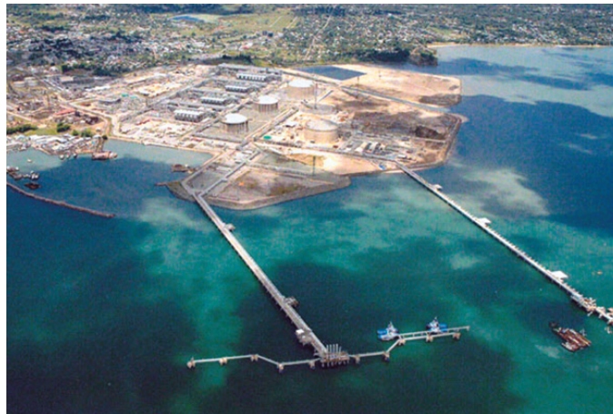
Atlantic LNG Plant located in Trinidad, including Chart liquefaction cold boxes and vacuum-insulated pipe for jetty cool-down lines
